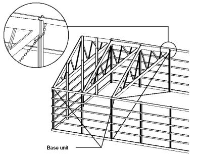
**Note:** Purlins, truss web restraint/bracing & some nailers omitted for clarity. Resist movement of the base unit perpendicular to the end wall with temporary ground bracing and/or chains or cables together with turnbuckles, or come-a-longs of sufficient strength. (min 2000lbs capacity) Provide a mechanical connection to resist truss rollover at the heel. This includes the use of nails, bolts, lag screws, metal straps or connectors per engineer of record. Top chord temporary
