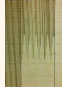
Finger-jointed and glued lumber resist individual ply separation and movement, assuring that every piece of lumber withstands warping and twisting.
