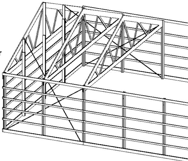
Provide a mechanical connection to resist truss rollover at the heel. This includes the use of nails, bolts, lag screws, metal straps or connectors per engineer of record.
